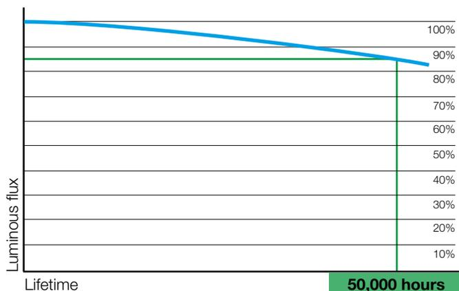
The percentage decline of the luminous flux with reference to the useful number of operating hours (usually 50,000 hours) is therefore determined with the parameter "L".
